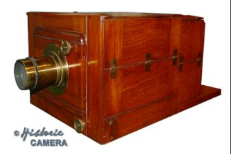
The Ottewill Wet Plate Camera was manufactured by Thomas Ottewill in London England in circa 1853. The Ottewill sliding box camera had a unique collapsible design enabled by hinges, which allowed for the front and back panels to be removed, and placed on the baseboard. Thus allowing the camera to be folded into a flat package for carrying. This is considered one of the first compact cameras made.
